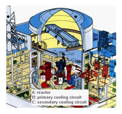
A cut-away view of the Japanese "Monju" fast breeder reactor. The two circuits contain sodium coolant with the secondary, non-radioactive loop drawing heat from the primary loop. The December, 1995 sodium leak occurred in the secondary circuit.
