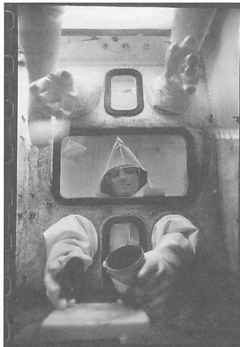
▲ Glove boxes are used to process plutonium because inhalation, even in tiny quantities, poses severe risks.
