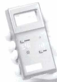
Portable survey meter (measures alpha, beta and gamma radiation)
