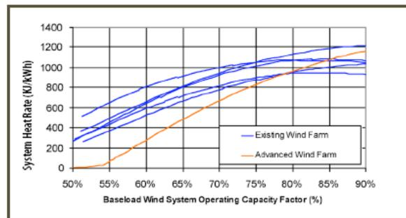
**Figure 5: Baseload Wind Plant Fuel Requirements**
