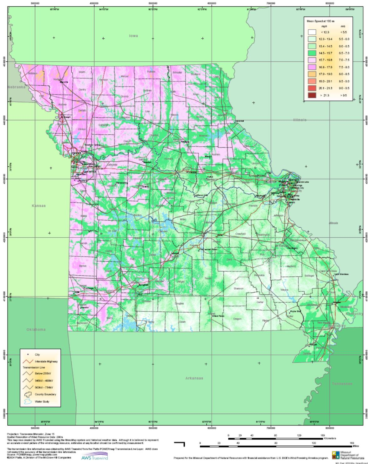
Figure 3: Missouri Wind Energy Potential at 100 meters
