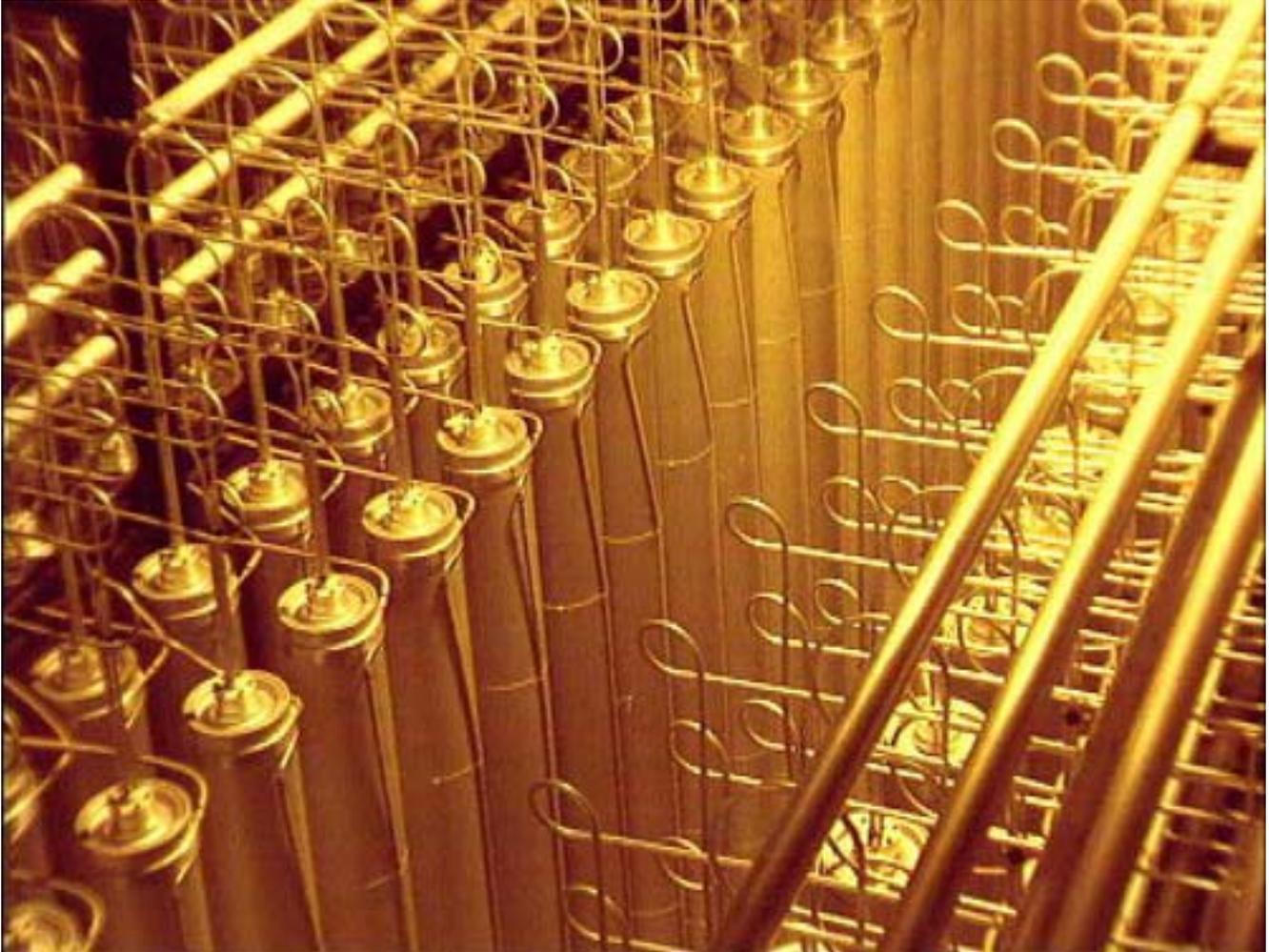
*Figure 5: A section of a typical cascade of centrifuge stages in a European uranium enrichment plant. The separative power of each centrifuge increases with the speed of revolution as well as with the height of the centrifuge while in a cascade each centrifuge also builds on the enrichment achieved in the previous stages. (photo taken from the Uranium Information Centre online at <http://www.uic.com.au/graphics/centrifge.jpg>)*
