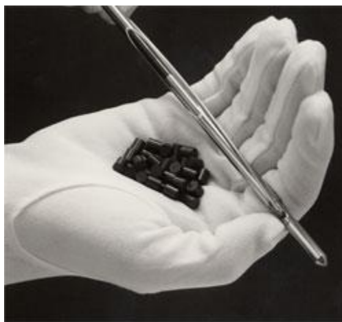
Figure 1: Fresh nuclear fuel pellets and a cutaway view of a fuel rod
