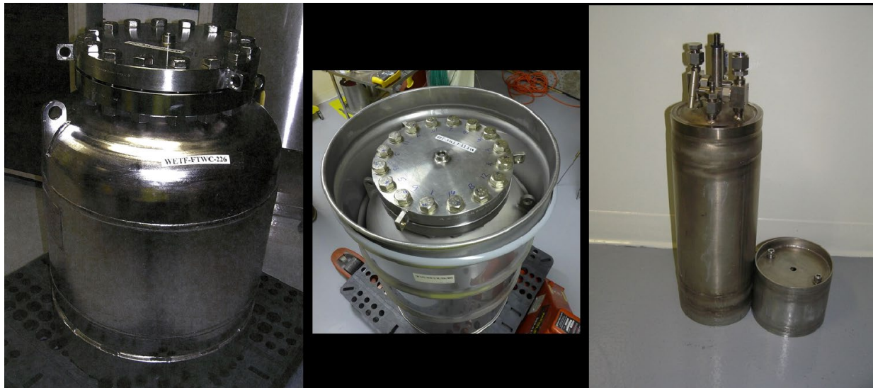
Figure 1: A FTWC is shown at left; an AL-M1 is at right. The center photo shows the FTWC stored in a larger barrel.
